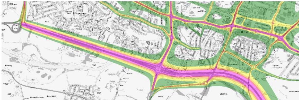
Figure 2 – Modelled NO 2 concentrations in the M4 AQMA (2014)
