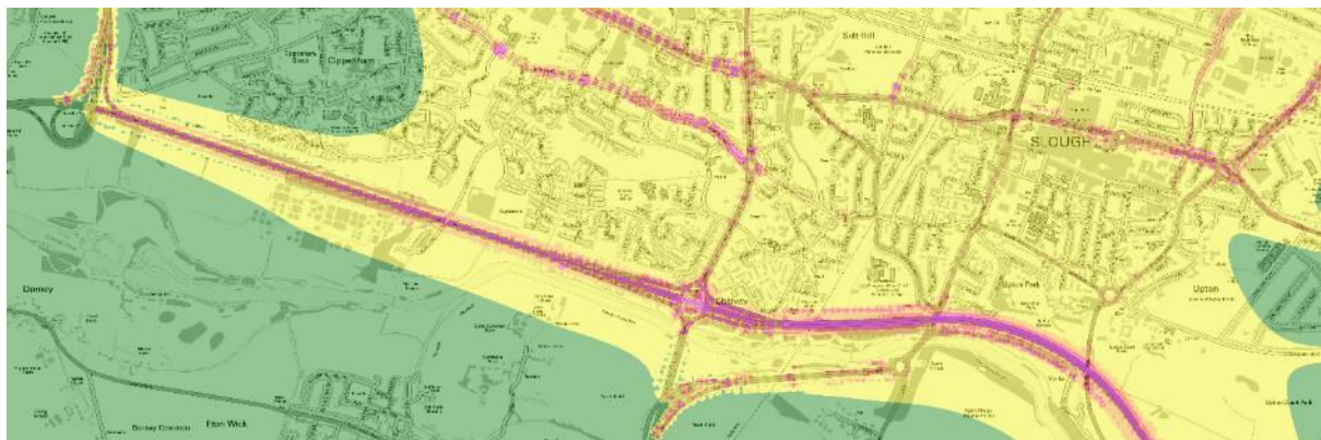
Figure 6 - Modelled PM2.5 concentrations for 2014 in the Town Centre, at Tuns Lane and along the M4
