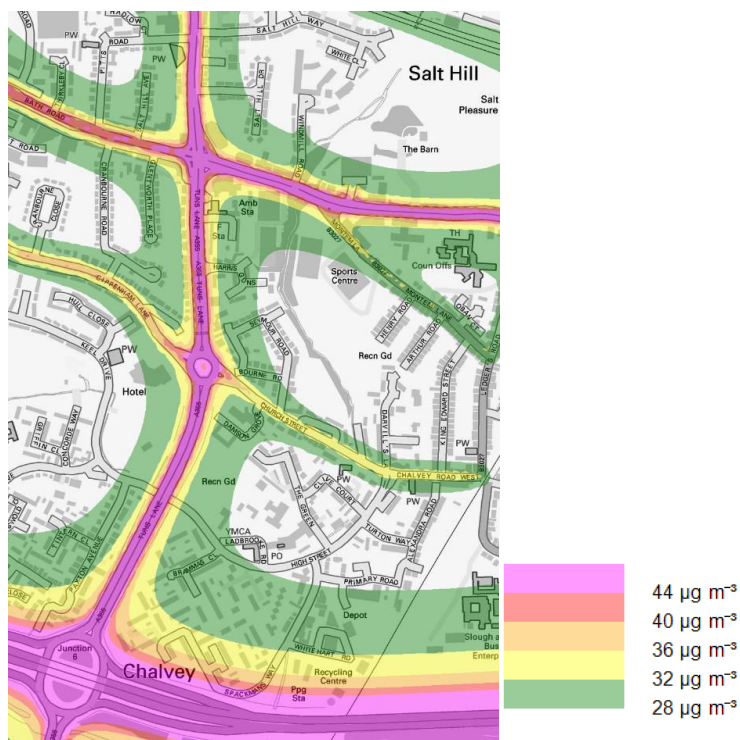
Figure 4 – Modelled NO 2 concentrations in the Brands Hill AQMA (2014)
